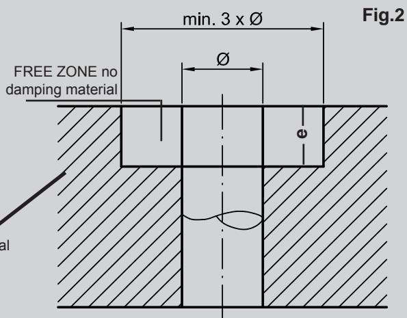
The dimension „e“ corresponds to the thread-free area of standard sensor types (-A21...). Otherwise „e“ is  $\geq 25$  mm.
