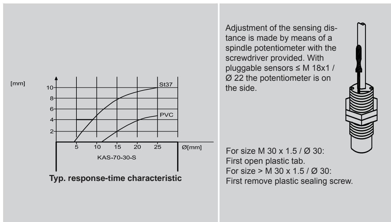
The possible sensing distance for a particular material is dependent on the dielectric permittivity  $\epsilon_r$  and can be worked out by means of the typical reduction factors:
