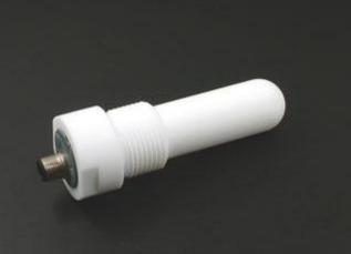
KA0655 KAS-80-26-A-PTFE-1"-Y5-StEx-N, ATEX PNP Non-Flush Mountable Normally Open or Normally Closed Process Connection: G 1 inch Y5 M12 Quick Disconnect connector PTFE housing with Metal
