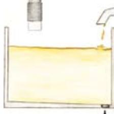
Overflow protection of casts, for example for plastic lenses for glasses with capacitive sensors of the KXS-Extreme series.
