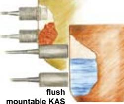
Detection of the content of a cardboard package e.g. tins with capacitive sensors (KAS)
