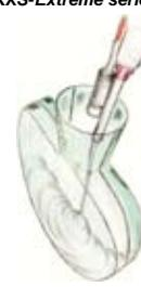
Detection of accumulations during the production of small parts with capacitive sensors of the KXS-Extreme series
