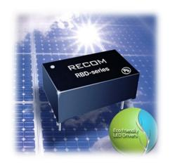
In summary, the RBD-12 series is able to boost the input voltage by a factor of 3. Therefore, it is possible to drive more LEDs in just one string. It also can increase the voltage of nearly depleted batteries. For this reason it is possible to ensure a constant performance even as the battery voltage decreases. The demand for buck-boost drivers like the new RBD-12 is growing - especially as the demand for solar-powered applications increases.
