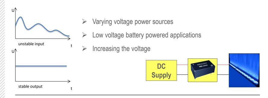
A boost converter is used with low voltage battery application to increase the voltage (for example, a solar powered application). This higher voltage is used for integrated circuits or longer LED strings that require this higher voltage. A boost converter may extract energy from a battery when the voltage is reduced due to a decrease in power. This voltage decrease occurs as batteries become depleted and is a characteristic of the ubiquitous alkaline battery.
