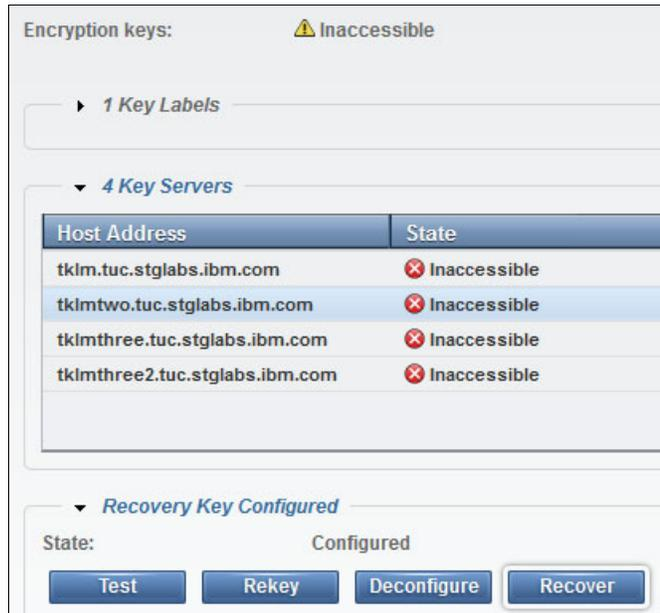
Figure 5-14 Start the recovery process
