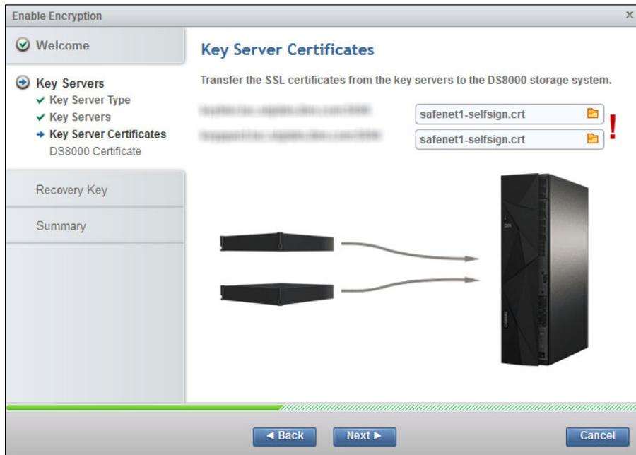
Figure 4-107 Transfer the SSL server certificate
