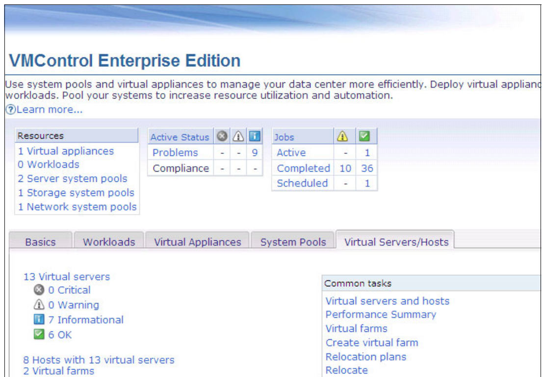
Figure 9-112 VMControl plug-in main window
