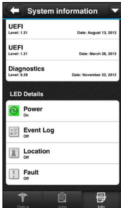
Figure 13-14 LED information as shown on the System Information window
