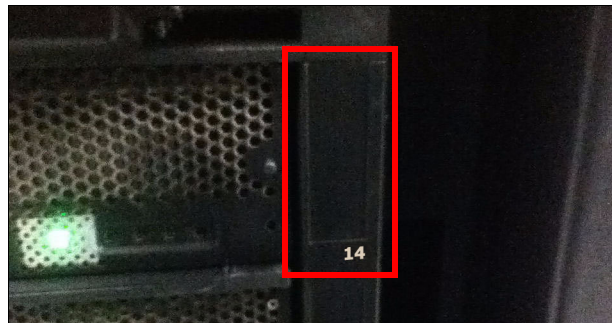
Figure 4-6 Chassis bay labeling
