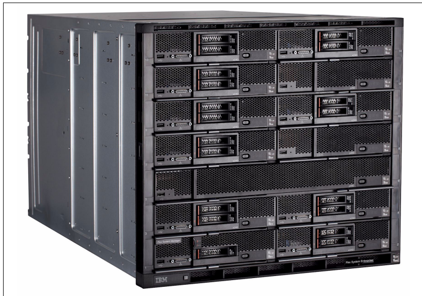
Figure 1-2 The IBM Flex System Enterprise Chassis
