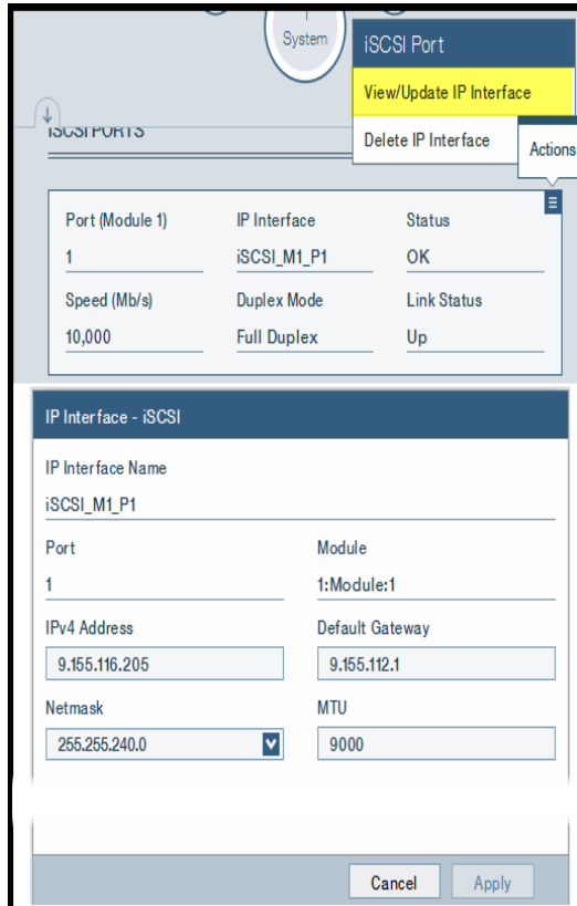
Figure 1-15 iSCSI Port properties displayed with Hyper-Scale Manager
