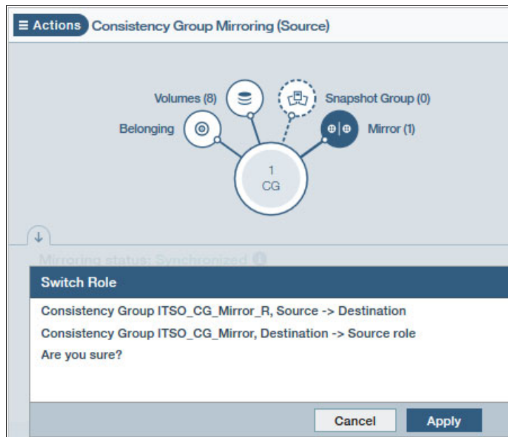
Figure 2-36 Switching the mirroring role
