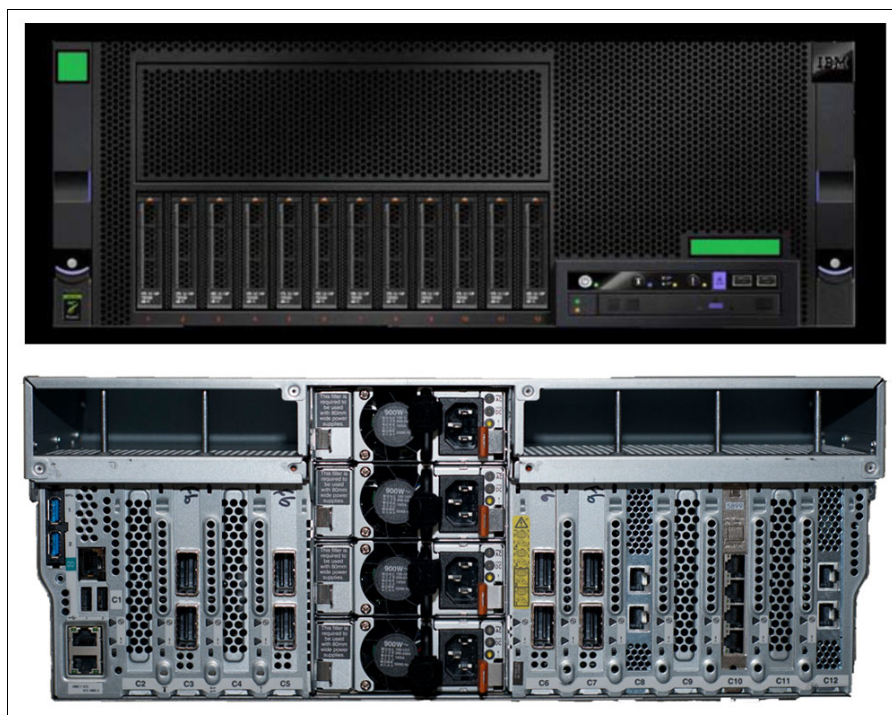
Figure 2-7 DS8886 processor complex front and rear views
