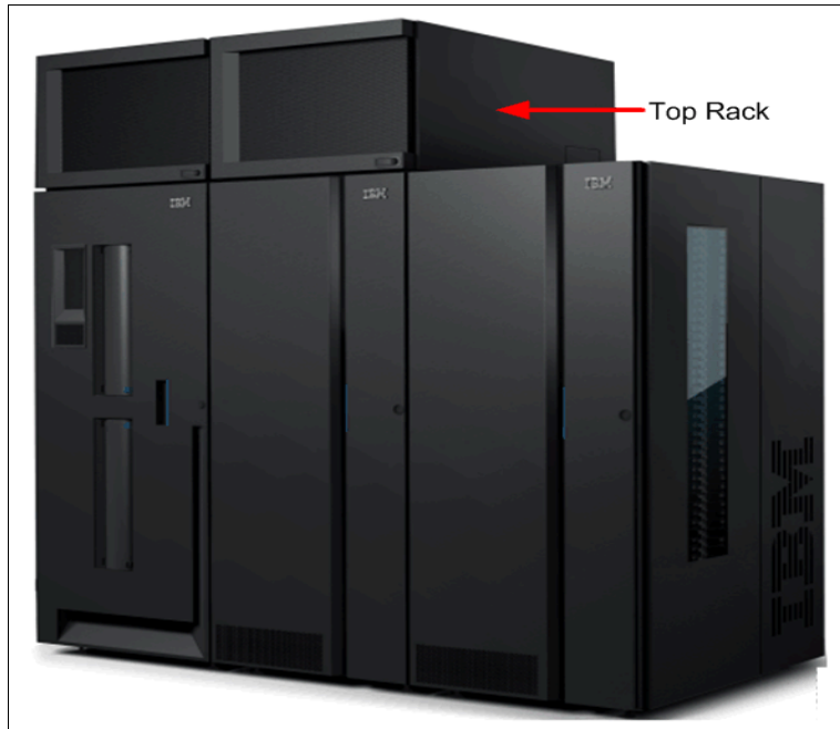
Figure 1-15 Tape library with an installed top rack
