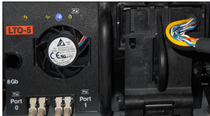
Figure 2-23 LTO-5 tape drive rear view
