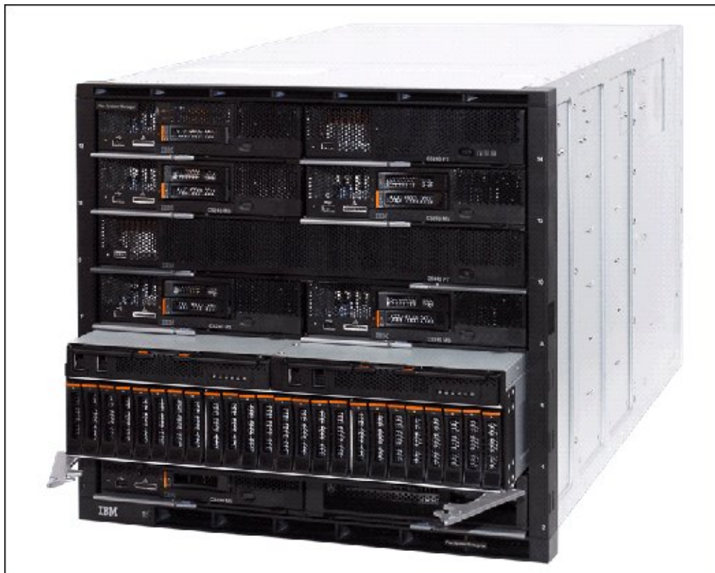
Figure 1. Front view of IBM Enterprise Flex System Chassis with IBM Flex System V7000 Storage Node
