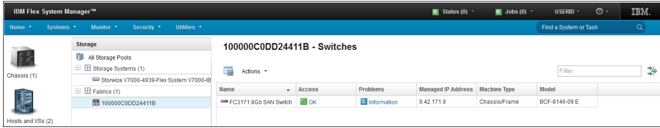
Figure 3-68 IBM FSM Explorer - Storage page - Switch overview
