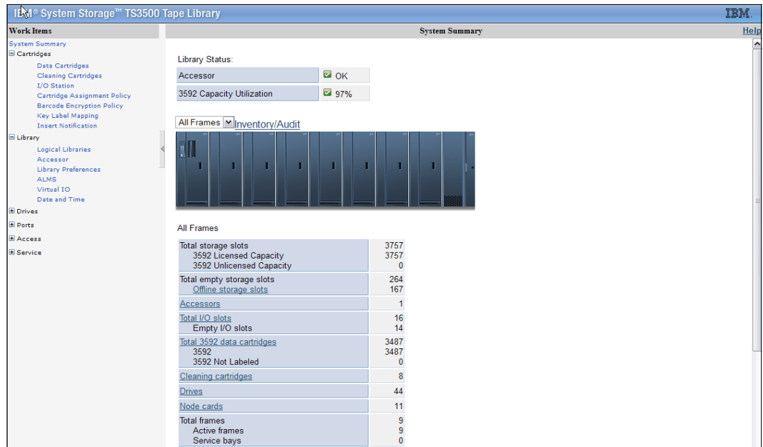
Figure 9-1 TS3500 tape library GUI initial window
