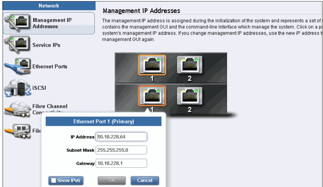
Figure 5-45 Viewing the management IP addresses
