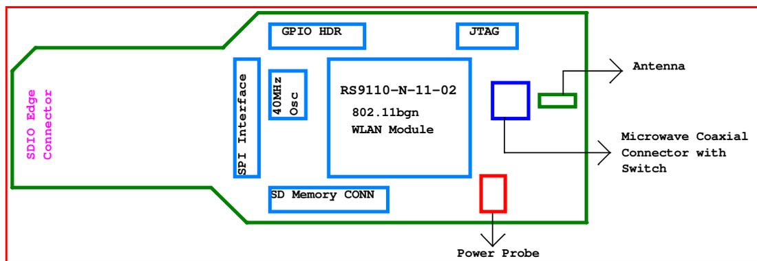
**Figure 1: RS9110-N-11-02 Evaluation Board Block Diagram**
