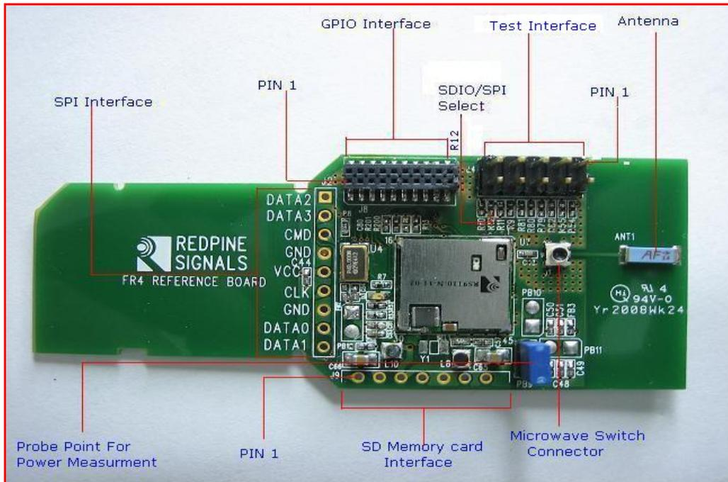
**Figure 2: RS9110-N-11-02 Evaluation Board and Connectors**
