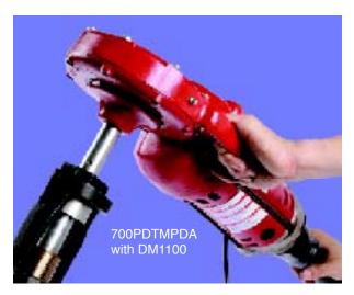
For Power Tapping with the 700PD Power Drive, the TMPDA (#08430) fits the 13/16" boring bar that is common on popular drilling and tapping machines. The operator manually turns the star feed on the tapping or drilling machine while the 700PD power drive adapter turns the boring bar. The 700PDTMPDA consists of the 700PD Power Drive and the TMPDA adapter.
