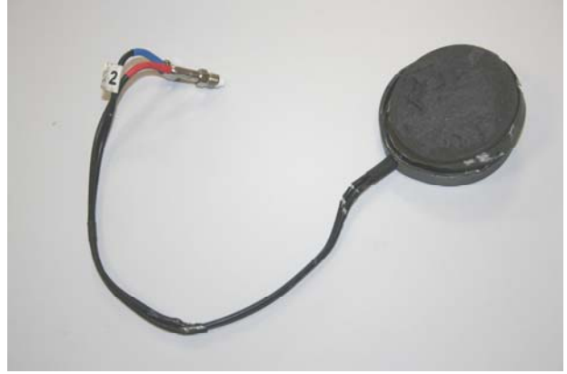
10: Broken cable on UUT 9 after vibration
