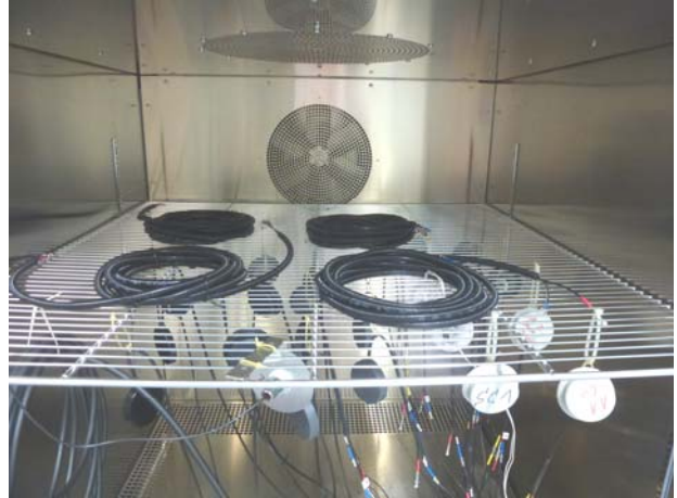
2: Cables in the climatic chamber
