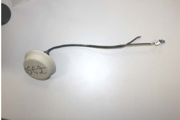
9: Broken connector on UUT 2 after vibration
