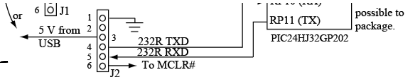
6-pin header for FTDI TTL-232R-3.3V USB-to-TTL cable (PC serial communication link)
