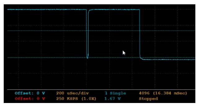
Mechanical switches can 'bounce' (cause multiple transitions) when pressed.
