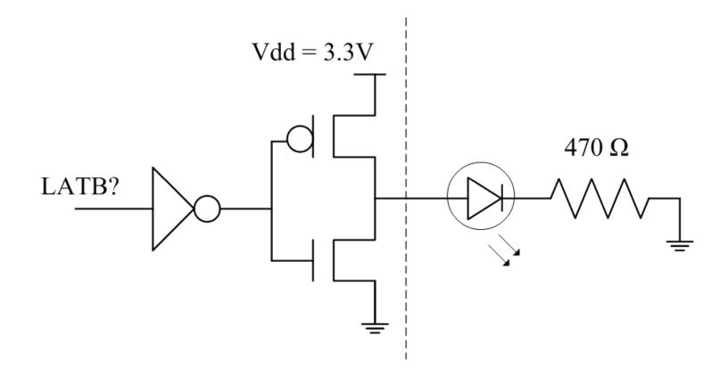
RB15/open drain configuration for heartbeat LED is a special case.
