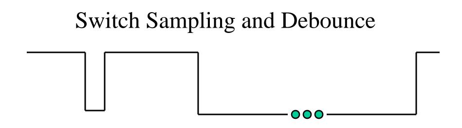
Our new approach is **periodically sampling** the switch every ~15 ms in our while(1) loop. In the first solution, we were reading the switch as fast as the cpu could loop.
