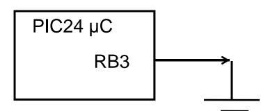
Configure RB3 as an open-drain output, then write a '1' to it.
