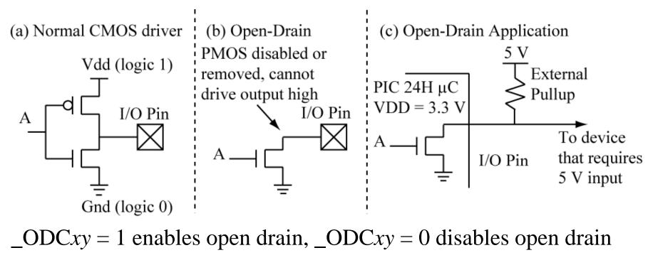
\_орсв15 = 1; Enables open drain on RB15
