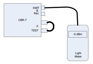
Disconnect the light meter from the transmitter. Connect the patch cable to the transmitter and all the other optical components. Measure the light level at the receiver of the corresponding CBR-7 repeater. This should be close to the level measured at the transmitter minus the calculated attenuation determined at design.
