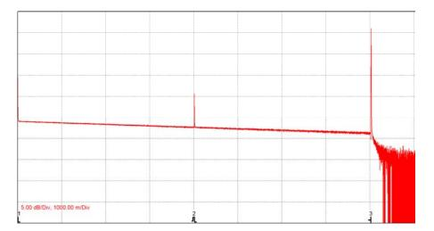
The top of the screen is at -10 dB. There are two reflections. One is at 4 km and the other at 8 km, at the end of the cable. The one at 4 km is 15 dB below the one at the end and it can be neglected since it is more than 10 dB below the reflection of interest at the end of the cable. The reflection at the end of the cable is at -14 dB. The return loss at the end of the cable due to this reflection is 14 dB, as seen from the other end of the cable where the measurement is made.
