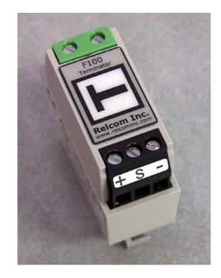
ditional ground connection will not cause ground loops. However, in the event of a voltage surge on the cable shield, a gas discharge tube in the **F100** fires and shunts this unwanted current to ground.
