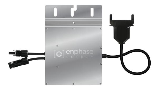
The Enphase® M250 Microinverter delivers increased energy harvest and reduces design and installation complexity with its all-AC approach. With the M250, the DC circuit is isolated and insulated from ground, so no Ground Electrode Conductor (GEC) is required for the microinverter. This further simplifies installation, enhances safety, and saves on labor and materials costs.
