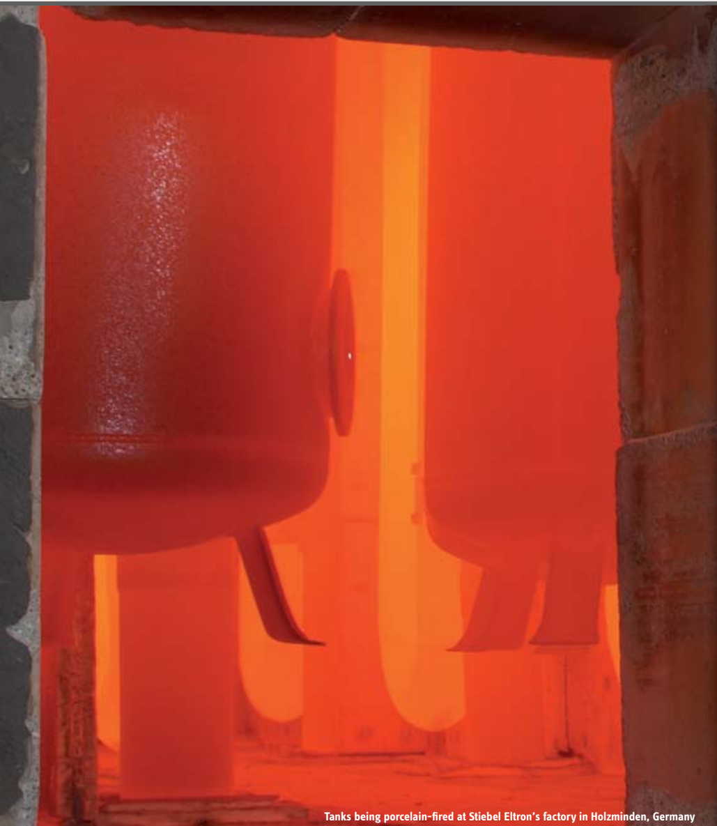
Tanks being porcelain-fired at Stiebel Eltron's factory in Holzminden, Germany
