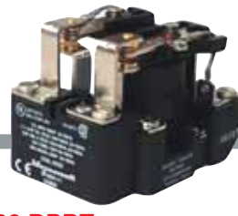
199 DPDT 40 AMP, 1-1/2 Hp PER POLE, 2 Hp-2 POLE SWITCHING
