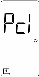
Loop Check Pending Indication
