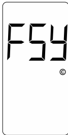
Parallel Synch Mode Failure Indication
