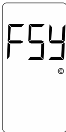
Series Synch Mode Failure Indication
