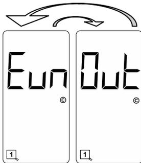
Uninitialized Motherboard Mounted EEPROM. The display will toggle between the two screens shown with a 50% duty cycle. This is an indication that the motherboard mounted EEPROM is uninitialized. To correct this problem, press the **FUNC** pushbutton. If the error message does not clear, the motherboard mounted EEPROM is defective. Return the detector to the factory for servicing.
