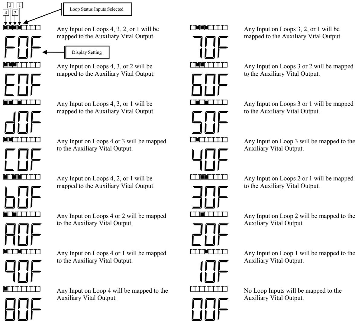
To set the mapping status of the Vital Input when in the Auxiliary Vital Output Mapping Program Mode, press the **CHAN** pushbutton once. The center character will flash indicating the current setting and the sixth bargraph segment from the left will show the corresponding Vital Input mapping. Use the ▲ (UP) or ▼ (DOWN) pushbutton to change the setting to the desired configuration. The two combinations of display characters and bargraph display are shown below.
