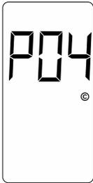
Upon application of power, the LCD screen will show the detector model letter and firmware version, in this case, Model P-1400 firmware version 4. This screen will be displayed for two seconds.
