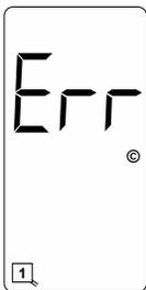
**Detection Reference Error.** This is an indication that the internal EEPROM and the motherboard mounted EEPROM detection reference values do not match. Press the **FUNC** pushbutton to clear the error message.
