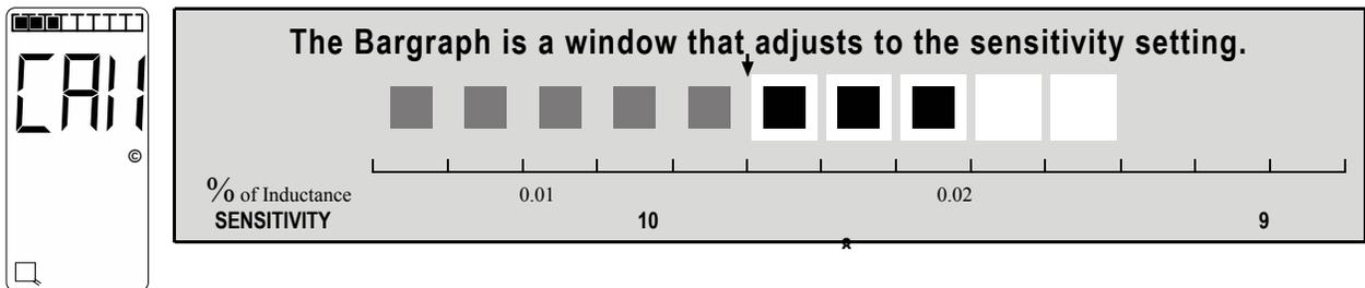
The bargraph below has the same vehicle in the loop zone causing the same inductance change as above. Because the sensitivity setting was increased to Level 8, six segments are now displayed. If the bargraph displays 5 or 6 segments for a vehicle in the loop, the sensitivity has been set to the proper range.
