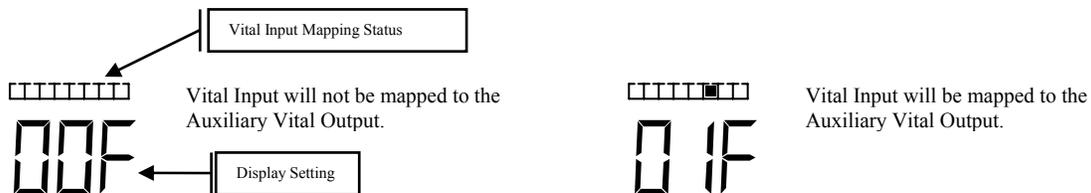
To set the mapping status of the Health Status Inputs when in the Auxiliary Vital Output Mapping Program Mode, press the **CHAN** pushbutton once again. The right character will flash indicating the current setting and the four rightmost bargraph segments will show the corresponding Health Status Input mapping. Use the ▲ (UP) or ▼ (DOWN) pushbutton to change the setting to the desired configuration. The various combinations of display characters and bargraph display are shown below.
