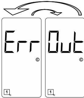
**Motherboard Mounted EEPROM Error.** The display will toggle between the two screens shown with a 50% duty cycle. This is an indication that the data stored on the motherboard mounted EEPROM is corrupt. Press the **FUNC** pushbutton to copy the reference data stored on the internal EEPROM to the motherboard mounted EEPROM. If the error message does not clear, the motherboard mounted EEPROM is defective. Return the detector to the factory for servicing.
