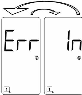
**Internal EEPROM Error.** The display will toggle between the two screens shown with a 50% duty cycle. This is an indication that the data stored on the internal EEPROM is corrupt. Press the **FUNC** pushbutton to copy the reference data stored on the motherboard mounted EEPROM to the internal EEPROM. If the error message does not clear, the internal EEPROM is defective. Return the detector to the factory for servicing.
