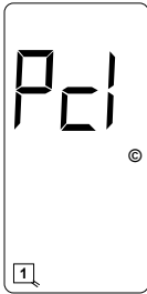
Loop Check Pending Indication
