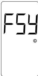
Parallel Synch Mode Failure Indication
