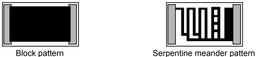
Figure 2. Block and serpentine meander pattern resistor elements.
