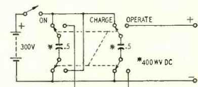
Fig. 5—A possible high-voltage source—using charged capacitors.
