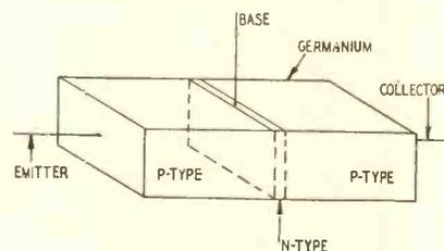
Fig. 1—A p-n-p junction transistor.
