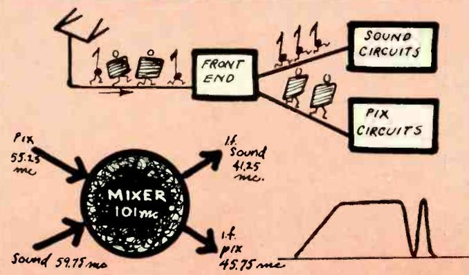
admit the whole band without attenuation, but the pix circuits have to keep the sound carrier and its sidebands out. So your selectivity curve must be flat and broad, yet have very steep sides. If not, you get sound mixed up with the picture. Then you really have trouble.
