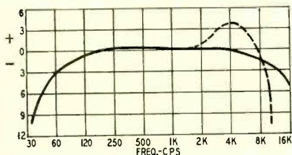
Fig. 1—Responsive curves. Solid line—authors circuit; dotted line—A.C.A.
