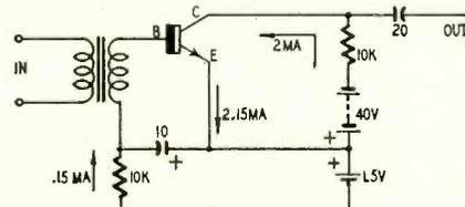
Fig. 4—Practical transistor hookup.
