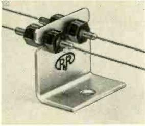
Uses for the IN35 are in FM discriminators, ratio detectors, phase detectors, industrial control circuits, and other applications requiring matched pairs of diodes.
