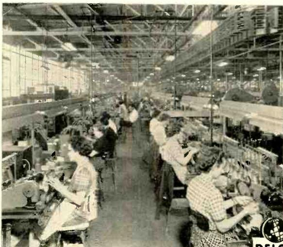
*Each RF and IF coil is wound under the supervision of a skilled operator, and each is tested at several points along the production line. This painstaking care is what gives a high IQ to Delco Radio Coils.*
