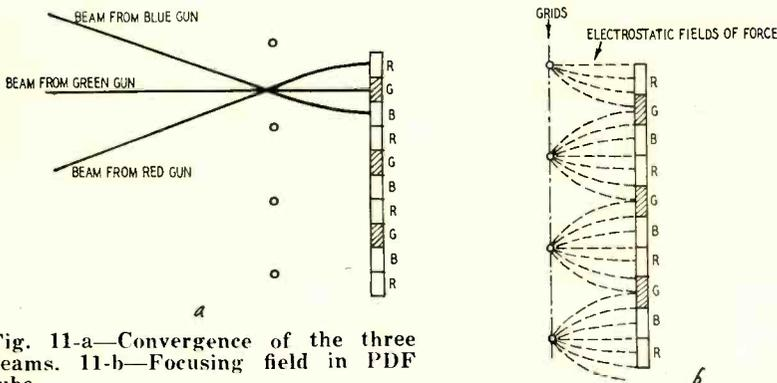
Fig. 11-a—Convergence of the three beams. 11-b—Focusing field in PDF tube.
