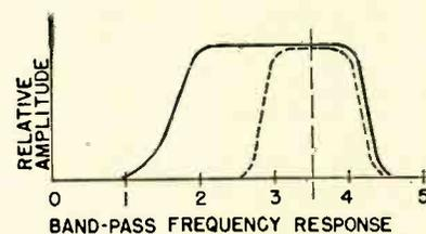
Fig. 4—Luminance channel pass-band.
