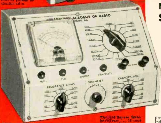
You will build the new Sprayberry 18-range Volt-Ohm-Milliammeter readings plus output meter and condenser and resistor substitution selector.
