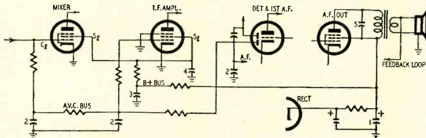
Fig. 1—Schematic shows several sections of a typical a.c. receiver.
