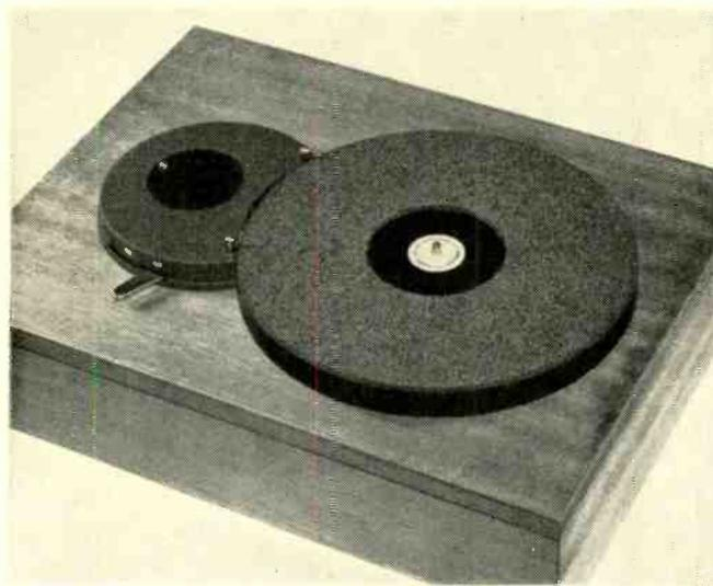
**Precision D & R turntable. Runout tolerance on table periphery is .001 inch.**
