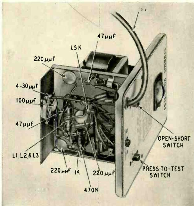
Instrument tests capacitors from 30  $\mu\text{f}$  to 2000  $\mu\text{f}$ .
