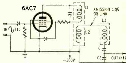
L2 feeds the harmonic to a series-tuned combination L3, C1, C2. The output voltage depends upon the Q of this output coil, so it should be as high as possible. C1, C2, form a capacitive divider which feeds the harmonic to the next stage.
