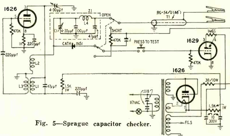
Fig. 5—Sprague capacitor checker.
