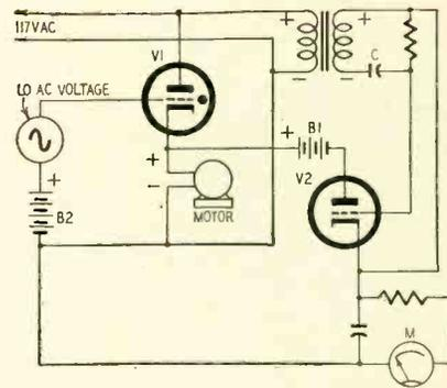
During the next half-cycle, V1 blocks and no current is applied to the motor. Of course this machine continues to turn over because of its inertia. During this time, counter-e.m.f. exists without applied voltage. The counter-e.m.f., like the applied voltage, is positive. It is fed to the plate of V2. Since the polarity has reversed, we find the grid of V2 is also positive, and this triode conducts. The meter deflects and indicates the magnitude of the counter-e.m.f. at the motor.
