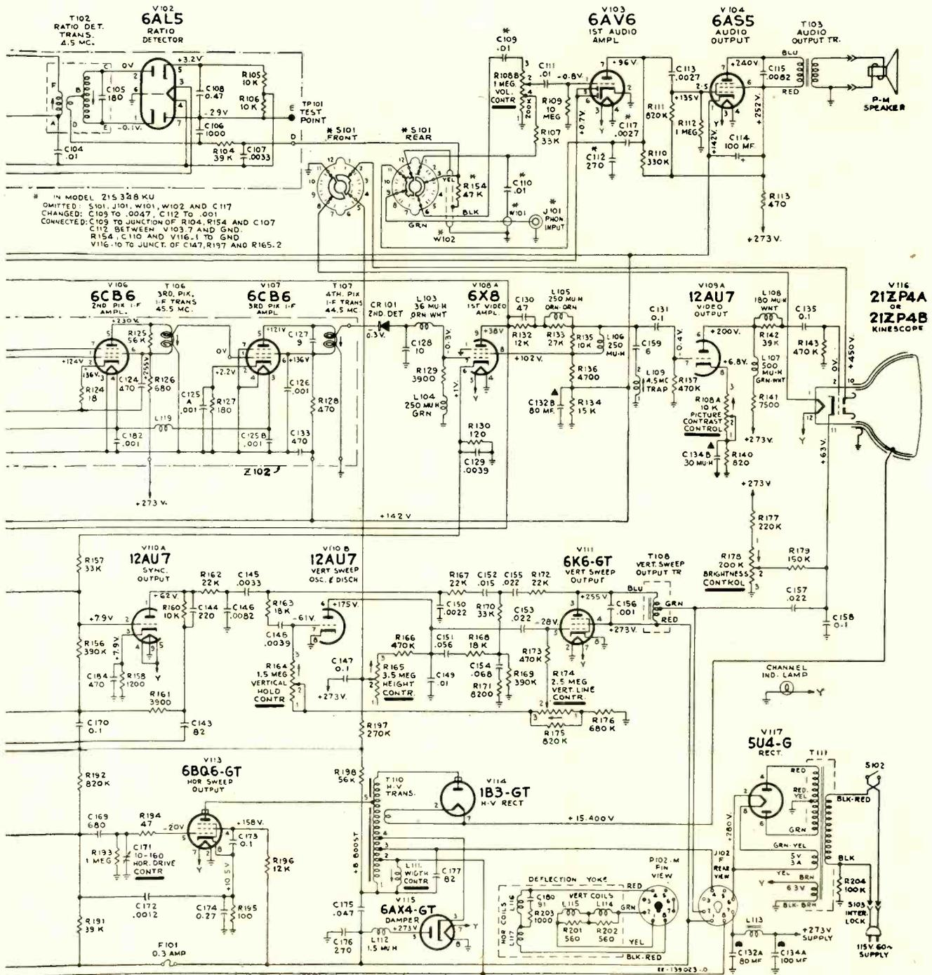
\* Chassis KCS88H is identical to chassis 88F except as noted on diagram.
