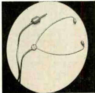
The high-fidelity range covers both speech and music. Its under-the-chin styling makes it suitable for use by women, eliminating hair muss and head-band fatigue. Its sensitivity is 105 db above .000204 dynes per square centimeter for 1 milliwatt power input, and the frequency range is from 50 to 8,000 cycles or better.
