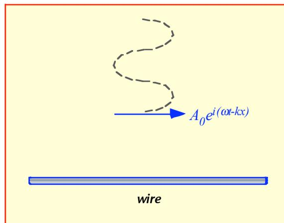
*Figure 1: wire and impinging potential; for simplicity,  $\mathbf{A}$  is taken along the axis of the wire and the direction of propagation is perpendicular to the wire.*
