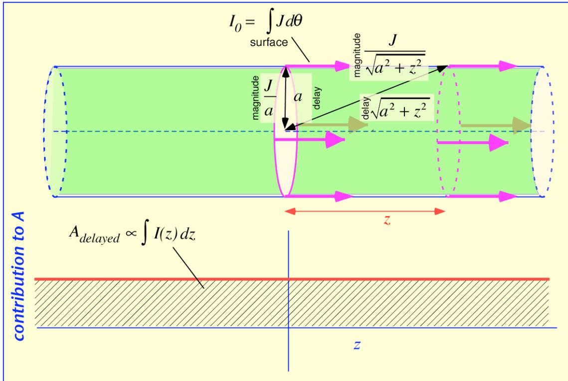
Figure 6: contributions to delayed vector potential along the axis of the wire; as long as the delay is small increasing delay compensated decreasing magnitude, so that all parts of the wire contribute equally.
