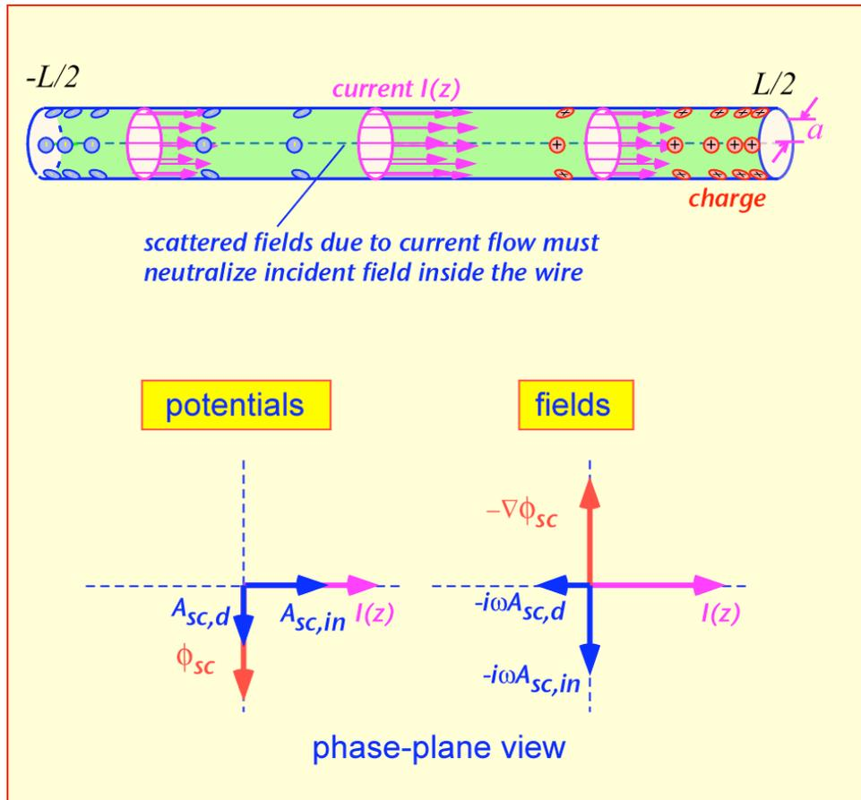
Figure 2: current and charge on the wire; resulting potentials and fields and their phase relationship with the current
