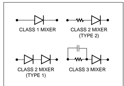
Figure 16. The various classes of mixers have different elements.
