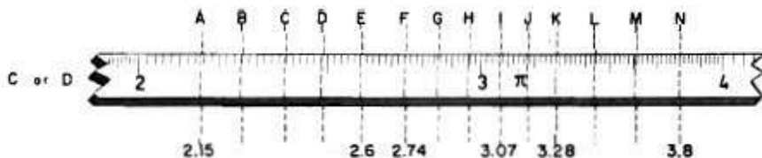
Fig. 10. Reading the portion of the C and D scales between 2 and 4.
