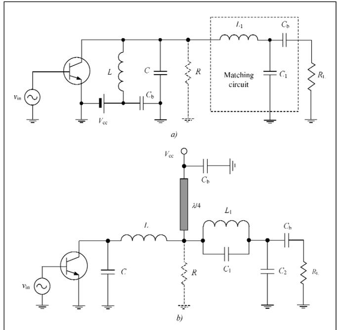
Figure 11 · Class E power amplifiers with a lumped element matching circuit.
