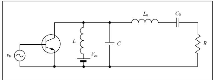
Figure 6 · Equivalent circuit of the parallel-circuit Class E power amplifier.
