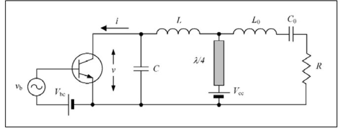
Figure 9 · Equivalent circuit of Class E power amplifier with quarter wave transmission line.
