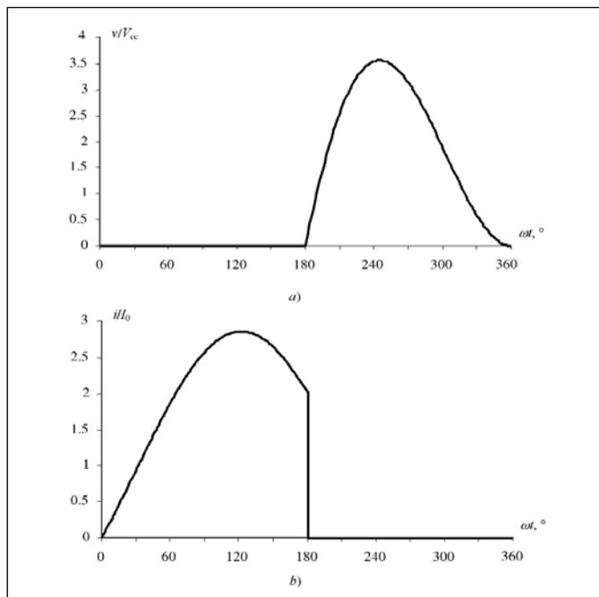
Figure 3 · Normalized collector voltage (a) and current (b) waveforms for idealized optimum Class E with shunt capacitance.
