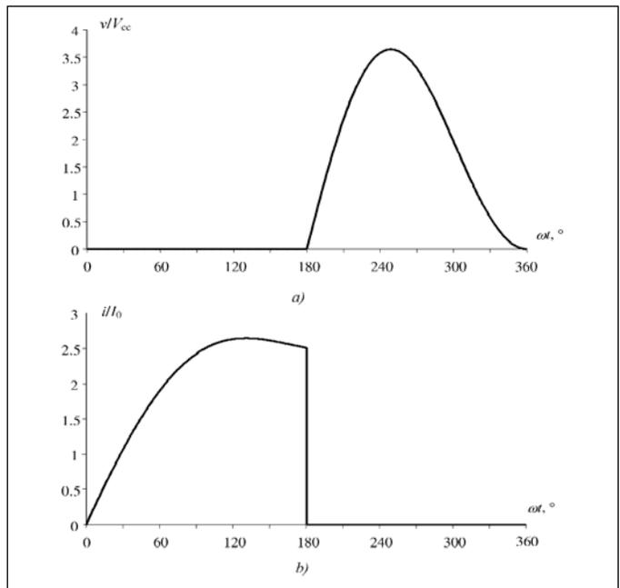
Figure 7 · Normalized collector voltage (a), and current waveforms (b) for an idealized optimum parallel-circuit Class E.
