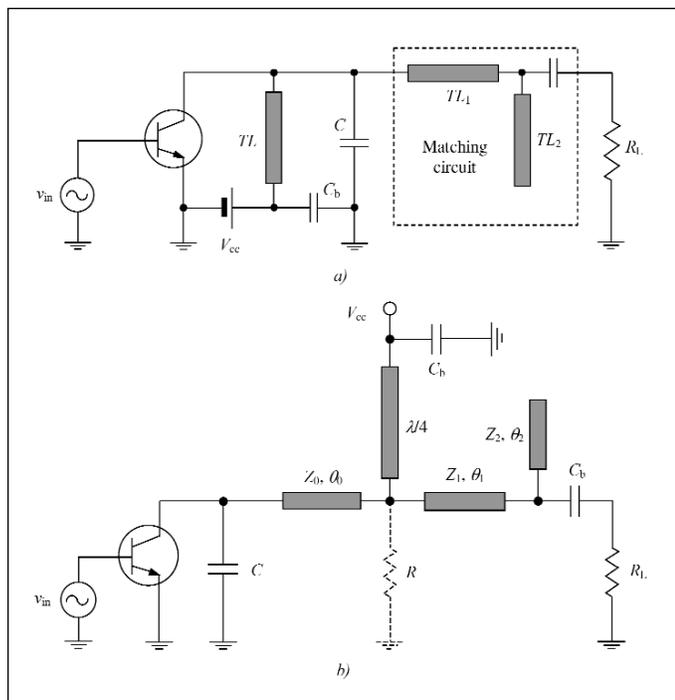
Figure 12 · Class E power amplifiers with transmission line output matching circuits.
