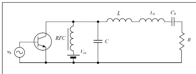
Figure 2 · Equivalent circuit of the Class E power amplifier with shunt capacitance.
