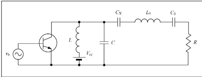
Figure 4 · Equivalent circuit of the even harmonic Class E power amplifier.
