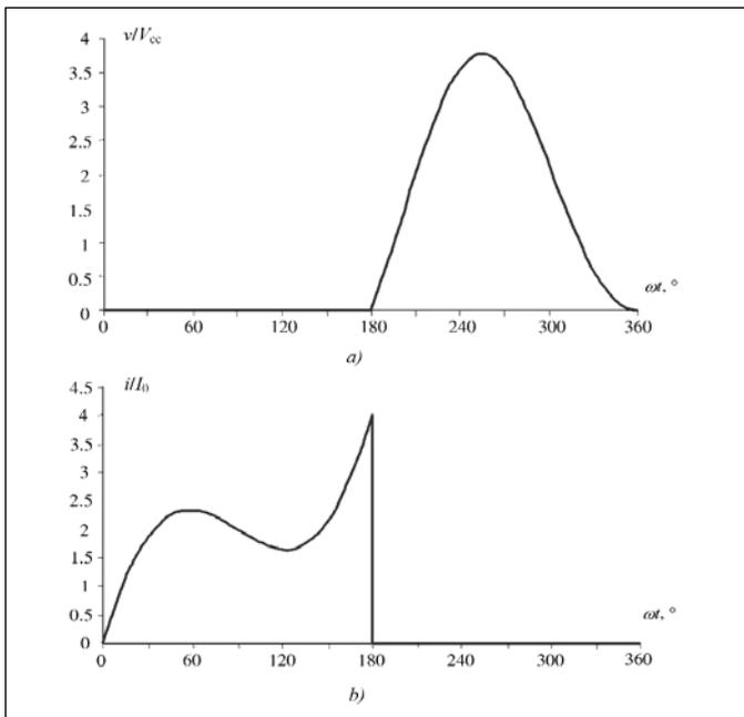
Figure 5 · Normalized collector voltage (a) and current (b) waveforms for idealized optimum even harmonic Class E.
