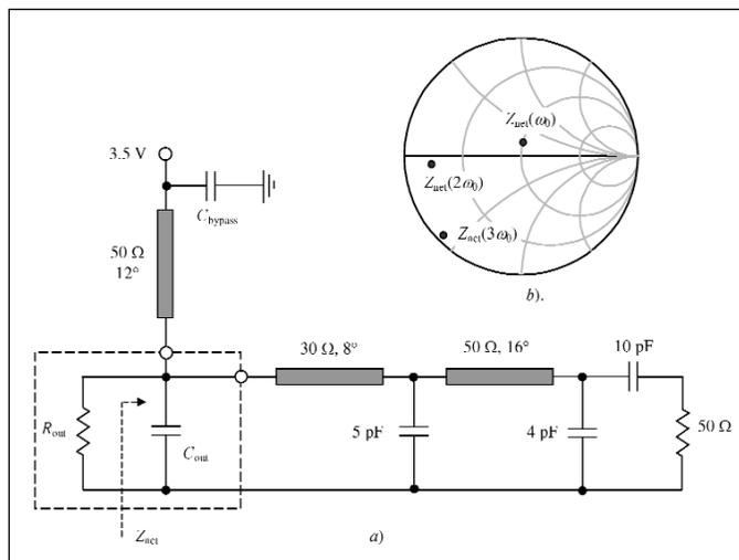
Figure 13 · Output load network of transmission line parallel-circuit Class E power amplifier for handset application.
