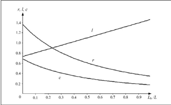
Figure 8 · Normalized optimum load network parameters versus normalized bondwire inductance  $L_b/L$  for parallel-circuit Class E.
