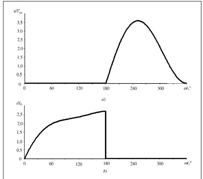
Figure 10 · Voltage and current waveforms of Class E power amplifier with quarter wave transmission line.
