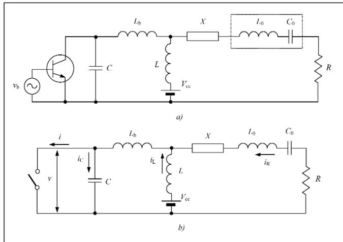
Figure 1 . Equivalent circuits of the Class E power amplifiers with generalized load network.
