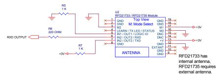
Every 2 seconds RXD will output the 5 bytes sent by the RFID transmitter, byte 1 will have bit 0 set to 1 to indicate that the source of the transmission was an RFID transmission, it will also have bit 4 set to 1 to which is the bit it forces high during an RFID transmission. The 4 following bytes, byte 2 through 5 will be the ESN of the transmitting RFID transmitter.
