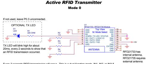
Every 2 seconds RFID transmission will occur. This is a dual-function mode, IN1, IN2, or IN3 if driven high will function exactly like they would in switch transmitter mode. IN1, IN2 and IN3 must all be kept low for RFID transmissions to occur automatically.
