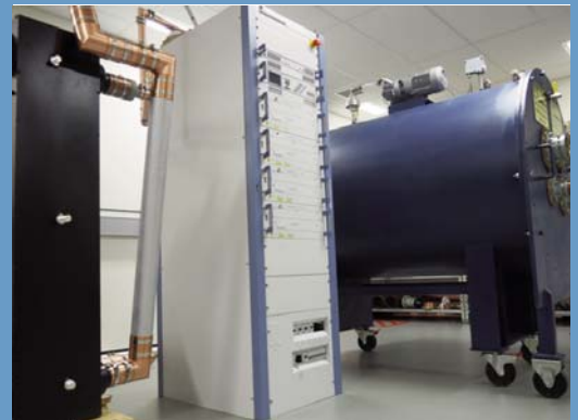
RFS FM test transmitter and low pressure chamber
