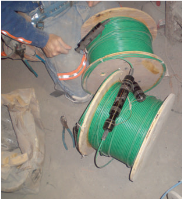
Most mines are using a military style connector, called a T-FOCA. (Photo courtesy of AFL)
