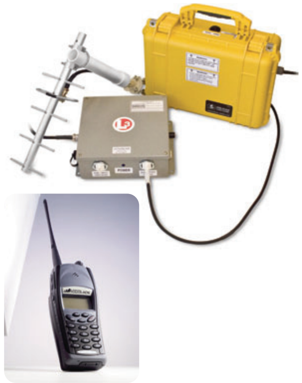
The L-3 ACCOLADE system transmits to the surface using a set of wireless nodes.
