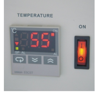
Heating device available for increasing tape adhesiveness.
