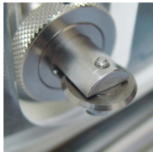
Heavy-Duty roller type harden steel cutter.
