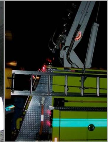
*Back lit version highly visible at night - meets FEMA regulations for fire apparatus.*
