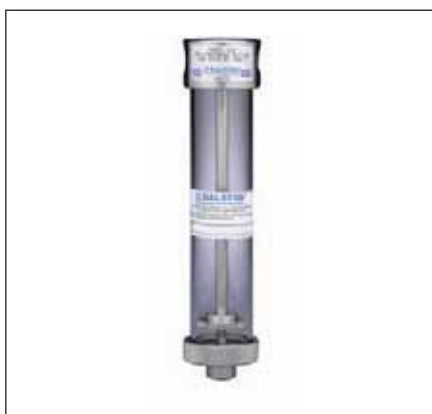
Figure 6 Model 95S6, 316 stainless steel with 5,000 psig pressure rating, is the filter housing most frequently used in process analyzers
