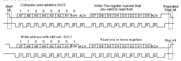
First send a start bit, the module address (0XC0) with the read/write bit low, then the register number you wish to read. This is followed by a repeated start and the module address again with the read/write bit high (0XC1). You now read one or two bytes for 8bit or 16bit registers respectively. 16bit registers are read high byte first. The compass has a 16 byte array of registers, some of which double up as 16 bit registers as follows;
