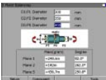
Show dual plane balancing data as a couple and a static one
