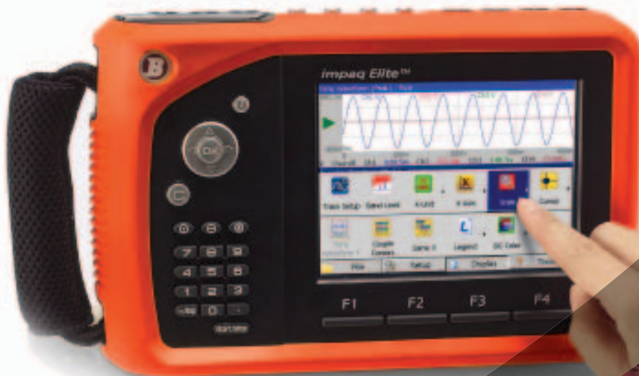
Display order spectral map, orbit and waveform, order spectrum and polar plot
