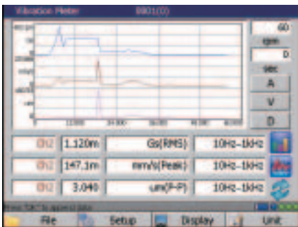
Measure and display overall level of acceleration, velocity and displacement in trend plot
