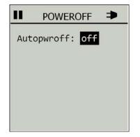
If this option is set, the instrument is switched off after the fixed time which has been set, from pressing any button. If it happened, the pressing of any button would cause the time count restart form zero.
