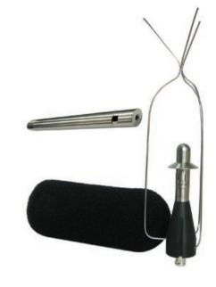
**OM231** is 1/2 inch prepolarized condenser outdoor microphone. It is suitable for use in rainy days or in an environment at very high or very low temperature. OM231 uses IEC 61672 CLASS 1 measurement microphone which is outstanding for its stability. It is the best choice for permanent outdoor use such as the airport noise monitoring.
