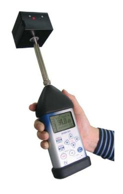
Sound Calibrator CA111 is a battery-operated sound source for quick and direct calibration of sound level meters and other sound measurement systems. It fits 1/2" microphones and 1/4" microphones with adaptors.
