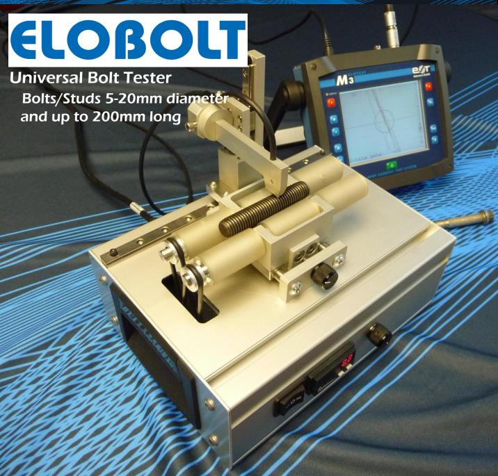
Areas of inspection: Thread and transition area between head and shaft Rollers easily adjusted to accommodate 5-20mm diameter bolts and studs Probe can be tilted to 45 degrees for transition area between head and shaft Speed adjustable from 0 to 200+ rpm in either direction
