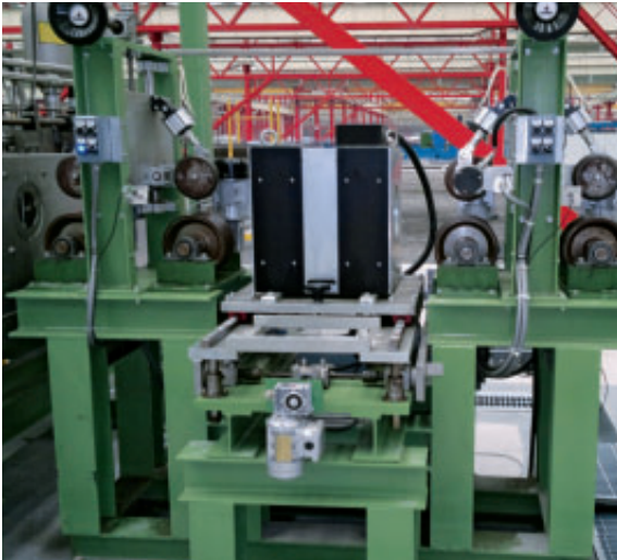
Inspecting wires / bars using encircling coils
