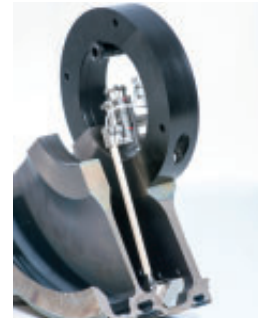
Manipulator-compatible probe, adapted for inspecting complex geometry
