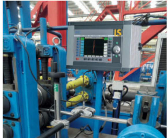
Testing the weld seam
