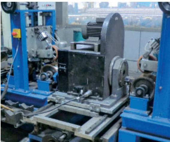
Bar inspection using EC100
