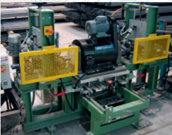
Steel bar inspection with EC100 rotor
