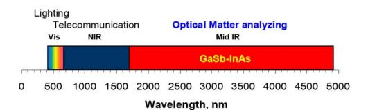
At the moment semiconductor optoelectronic devices for near-infrared and visible spectral range are widely used in telecommunications and lighting. In addition to these applications, LEDs and PDs posses great potential for using in optical analyzing systems.
