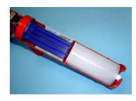
Place the filled adapter in the caulking gun barrel, aligning the plunger with the cartridge
