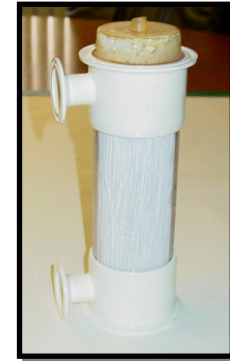
Reverse Osmosis Filter
